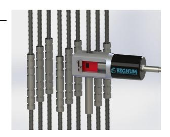
Prescoup cold-swaged Couplers are designed to splice bars in situ. A hydraulic swaging press with special dies deform the sleeve around the ends of the bars to be spliced. This method creates a mechanical connection
