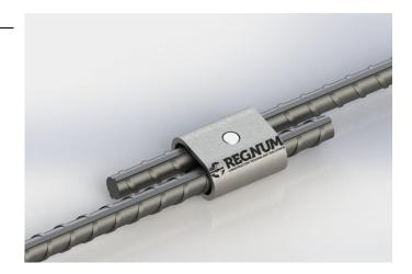
Fastcoup Couplers consists of an oval shaped steel sleeve and a wedge pin. The sleeve is placed around two steel bars that overlap. The wedge pin is placed on the sleeve and inserted into a handheld hydraulic pin driver. The pin is then driven to complete the connection through the pre-drilled hole in the sleeve and between the bars. In seconds, a pin is driven.
