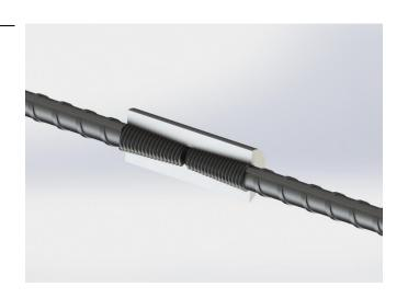
Tapercoup Couplers are designed to splice the same diameter bars where at least one bar can be rotated and moved freely in its axial direction. The couplers are machined to have taper threads inside which create a mechanical connection of two corresponding reinforcing steel.
