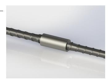
Barcoup Couplers are designed to splice the same diameter bars where at least one bar can be rotated and moved freely in its axial direction. The couplers are machined to have parallel threads inside which create a mechanical connection of two corresponding reinforcing steel.
