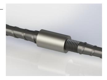
Barcoup L Couplers are designed to splice the same diameter bars where none of the bars can be rotated. The couplers are machined to have parallel threads inside which create a mechanical connection of two corresponding reinforcing steel.
