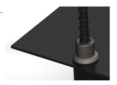
Weldcoup Couplers are designed to provide a fast connection between reinforcing steel bar perpendicular to structural steel sections and plates. These couplers are machined from weldable steel grades in order to facilitate simple welding process. Typical applications include connecting rebar to structural steel columns and beams. Structural integrity is established by welding before pouring concrete.
