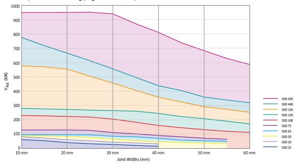
Regbar SSD  $V_{Rd}$  Design Resistance (kN) for Various Joint Widths (mm) at the Maximum Slab Thickness (mm) in C30/37 Concrete (See the following pages for details)
