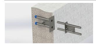
The two-part assembly of all Regbar shear connectors eliminates the need for drilling formwork on site, supporting dowel bars and fitting debonding sleeves and end caps. The installation is a fast and accurate process.
