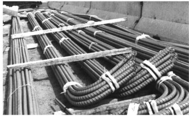
Fig. 5.1—Epoxy-coated reinforcing bar (courtesy of Concrete Reinforcing Steel Institute).
