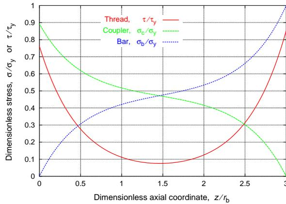
Fig. 10 Stress distributions for one half of a threaded coupler
