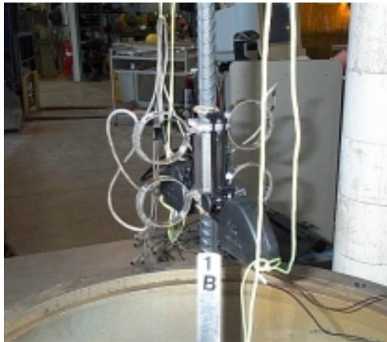
**Fig. 7 Test set-up for measuring end slips and extension over coupler**
