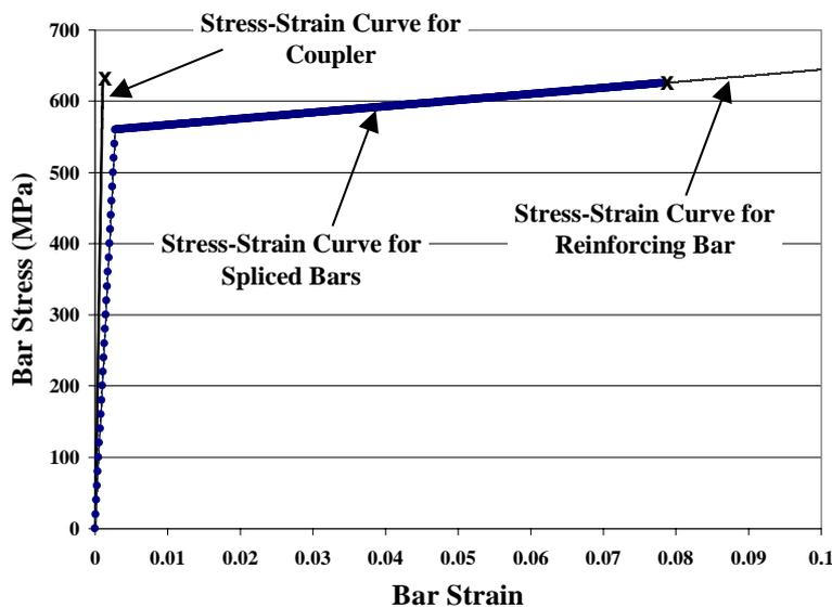
**Fig. 8 Effect of premature failure of coupler on spliced bar ductility**
