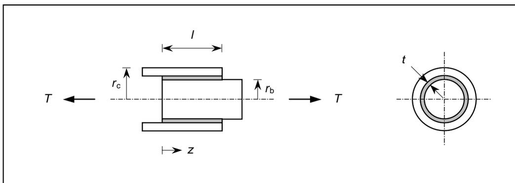
Fig. 9 Idealised theoretical model for one half of a threaded coupler
