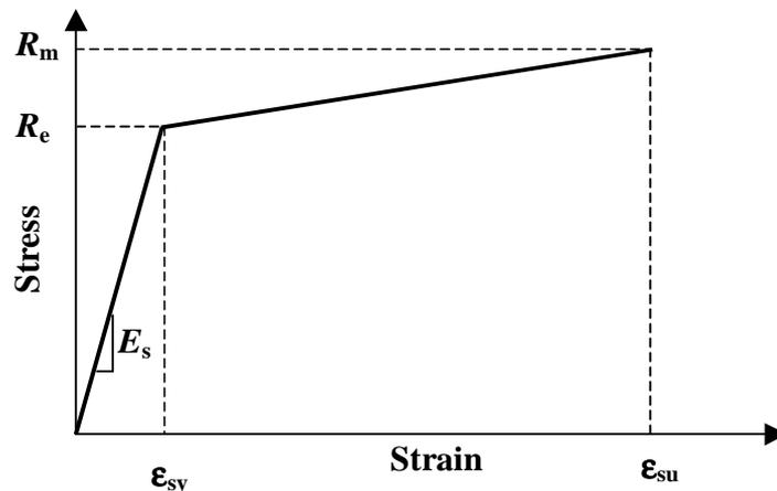
Fig. 3 Approximate stress-strain curve of new Australian 500N bar [3,6]
