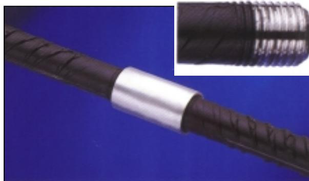
(a) Tapered thread cut into bar [8,9]      (b) End of bar forged, then threaded [10]
